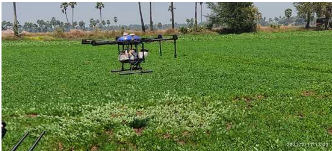
Figure 1. An UAV spraying of recommended chemicals for bio-efficacy and phytotoxicity studies
