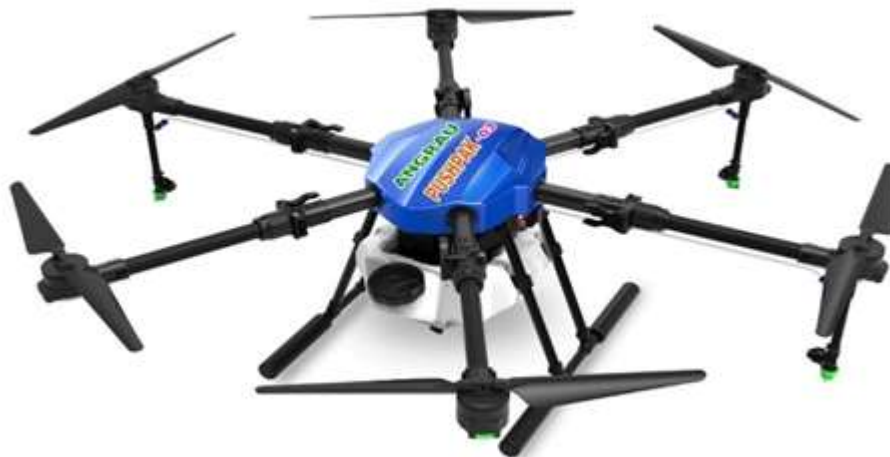
Figure 2. ANGRAU-PUSHPAK 01: An UAV standardized for agricultural spraying
