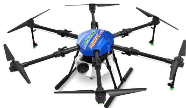
Figure 2. ANGRAU PUSHPAK-01; An UAV standardized for agricultural spraying.
