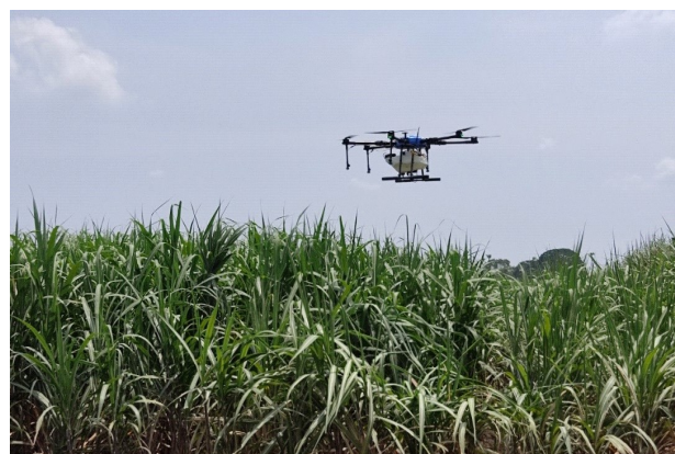
Figure 1. An UAV spraying of recommended chemicals for bio-efficacy and phytotoxicity studies
