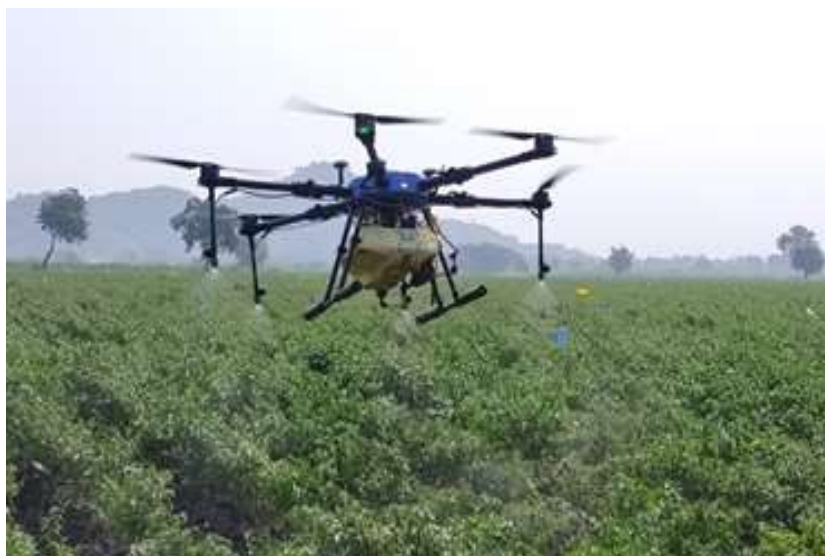
Figure 1. UAV spraying of recommended insecticides for bio-efficacy and phytotoxicity studies
