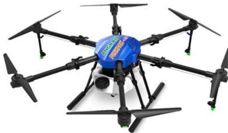
Figure 2. ANGRAU-PUSHPAK 01: An UAV standardized for agricultural spraying
