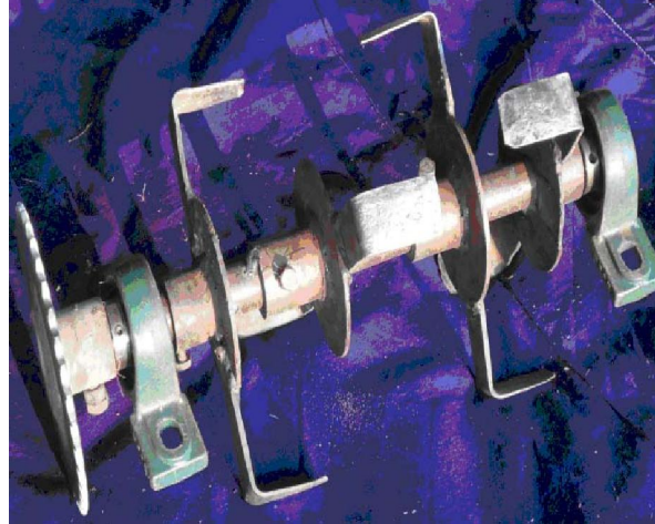
Fig 2. Assembly of L-blade rotor and sprocket arrangement
