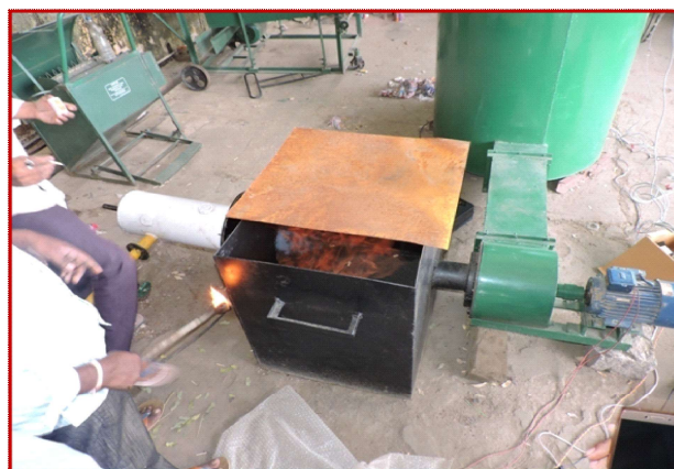
Fig 2. Paddy dryer coupled with gasifier
