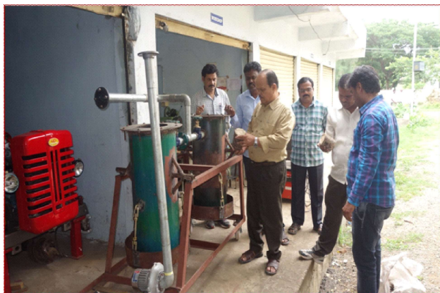
Fig 1. View of developed gasifier for heat supply
