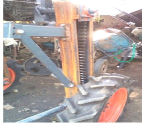
Fig 2. Arrangement of chain and sprockets for rear wheels
