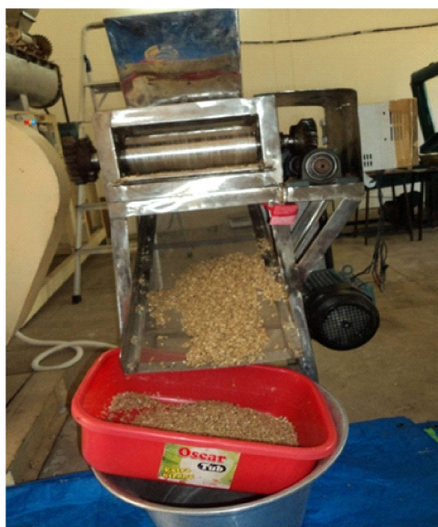
Fig 2. Developed sorghum roller flaking machine in operation
