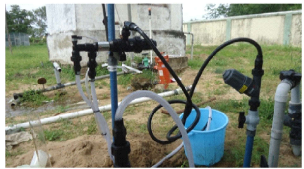
Plate 3. Experimental set up of fertilizer injection pump
