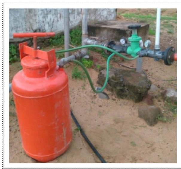
Plate 2. Experimental set up of Fertilizer tank assembly
