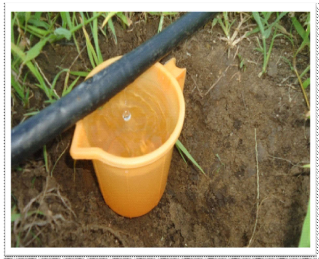
Plate 4 Collection of discharges for uniformity coefficient determination
