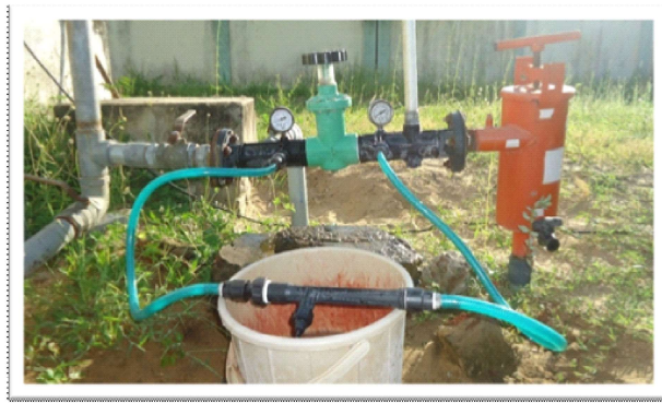
Plate 1. Experimental set up of venturi injector
