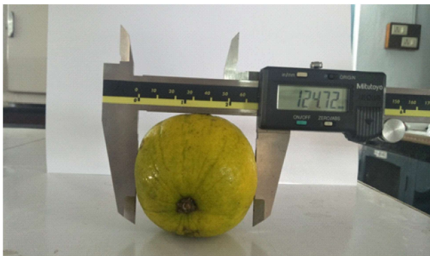
Plate 1. Measurement of linear dimensions using digital calipers
