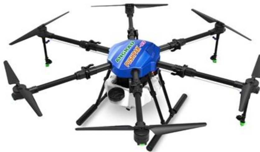
Figure 1. ANGRAU-PUSHPAK 01: An UAV standardized for agricultural spraying
