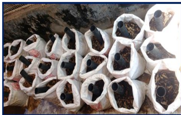
Fig 1. Composting experiment with a combinations of aqua sludge + rice straw (9 bags on the left) and aqua sludge + water hyacinth (9 bags in middle), aqua sludge + paddy straw + water hyacinth (6 bags on right) and aqua sludge alone (control- 1 bag).
