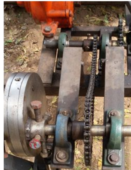
Plate 2. Final reduction transmission system (Chain and sprocket) used in punch planter
