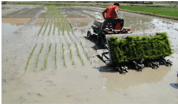
Fig 1. Testing of 4WD tractor mounted paddy transplanter under actual field condition
