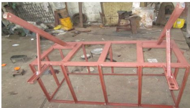
Fig. 3. Chemical tank holder fitted to the tractor
